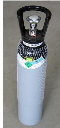
A typical nitrogen cylinder
