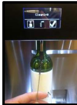
Step 6: Use the **Brush to clean the nozzle** and **repeat Step 5** until the bottle is empty
