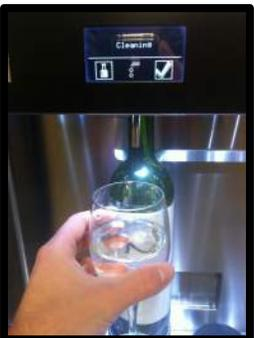
Step 7: Press the **right button**
