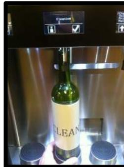
Step 4: **Place the cleaning bottle** filled up with hot water and citric acid (4 tables spoons or 2 oz ) on the piston and Press the **left icon**
