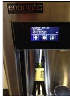
Step 4: Insert the **bottle straw** inside the new bottle and place bottle on the lifter. Select **change bottle** (the bottle will raise and seal against tap).
