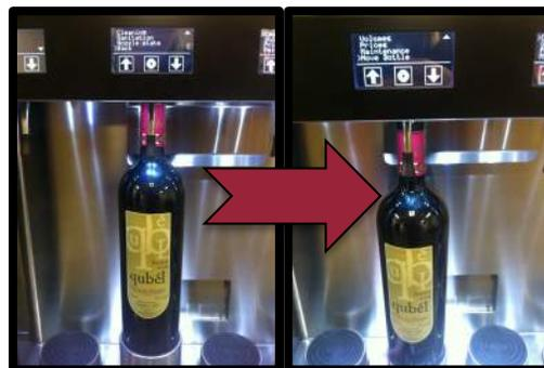
Step 8: **Place your wine bottle on the lifter**, then scroll down choose the option **back** and scroll down again to **move bottle.** Remove the **Tech card**
