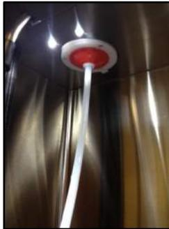
Step 3: Insert the **bottle straw** (Push straight up until firmly in place).
